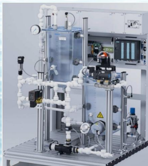
Figure 2. liquid pumping control MPS station
