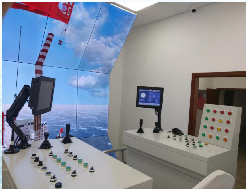
Figure 4. Hoisting operation simulator with 9 channels display
