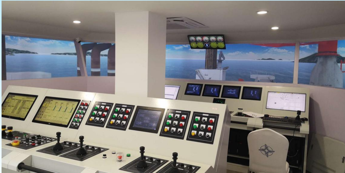
Figure 3. Main own ship system with 5 channels projection display
